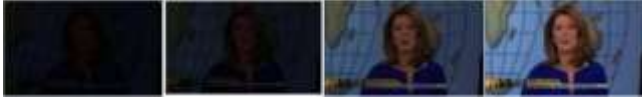
Shot A Gradual transition shot boundary Shot B Fig.4. Gradual shot boundary (dissolve transition)
